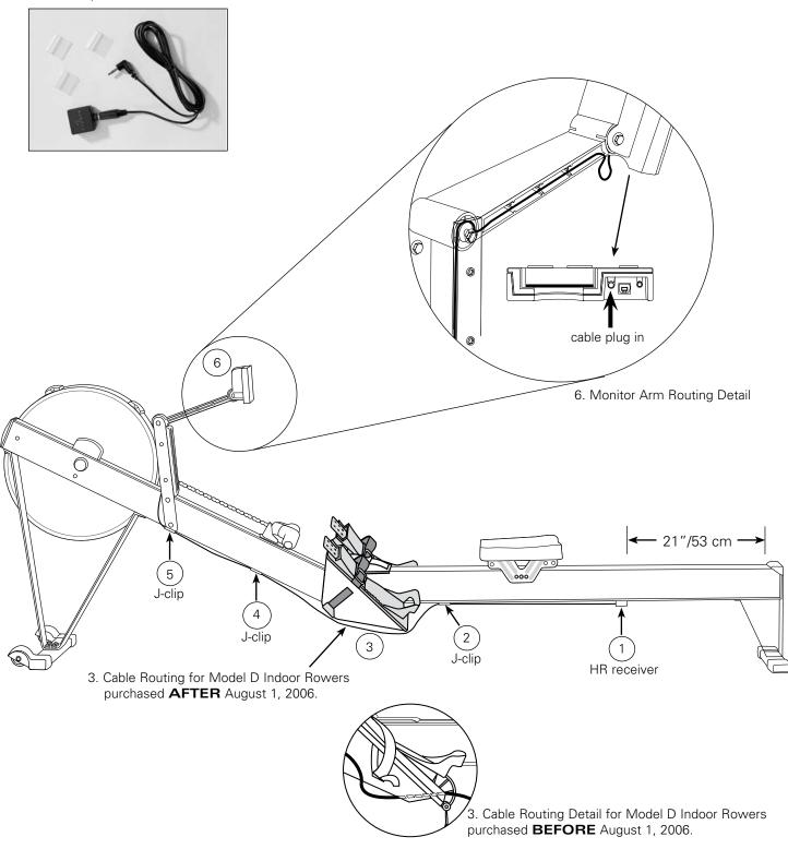
**NOTE FOR STORAGE:** Before disconnecting monorail from front end, remove receiver from VELCRO<sup>®</sup> patch and remove cable from framelock area.
